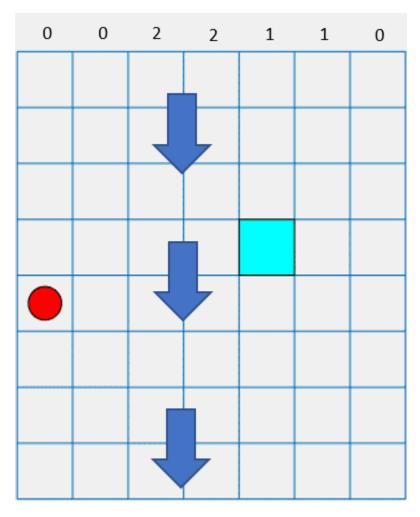
The intensity of the waterfall varies between the columns, as shown at the top of the preceding figure. When the agent moves into a column with a nonzero intensity, the waterfall pushes it downward by the indicated number of squares. For example, if the agent goes East from state [5,2], it will reach state [7,3].
