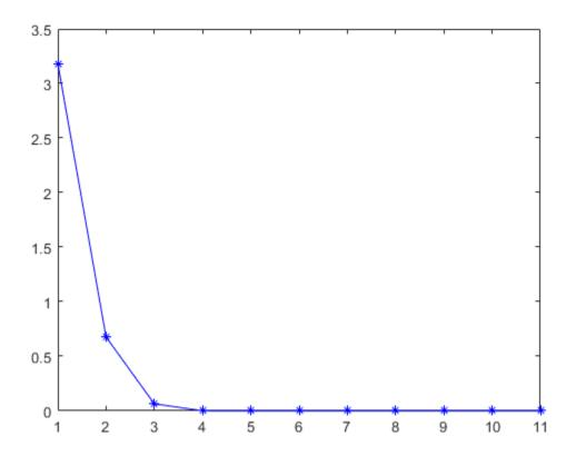
Compute the norm of final error for the feedback gain.
