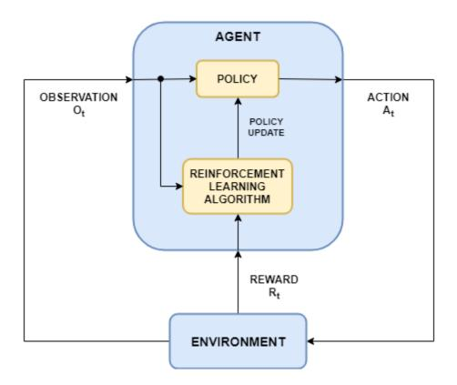
The goal of reinforcement learning is to train an *agent* to complete a task within an unknown *environment*. The agent receives *observations* and a *reward* from the environment and sends *actions* to the environment. The reward is a measure of how successful an action is with respect to completing the task goal.
