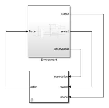
In the Enviornment subsystem, the model dynamics are defined using Simscape components and the reward and observation are constructed using Simulink blocks.
