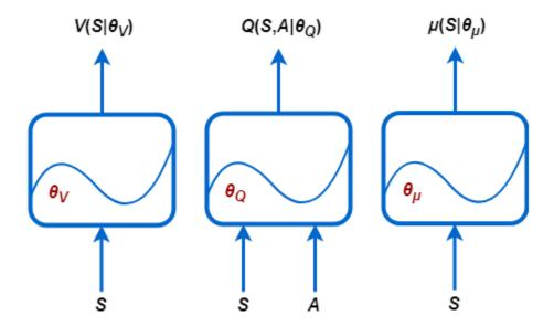
For systems with a limited number of discrete observations and discrete actions, you can store value functions in a look-up table. For systems that have many discrete observations and actions or with observation and action spaces that are continuous, storing the observations and actions becomes impractical. For such systems, you can represent your actors and critics using deep neural networks or linear basis functions.
