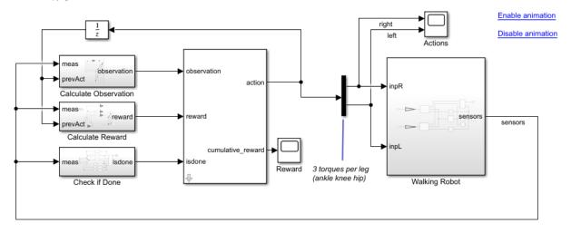
The robot is modeled using Simscape Multibody and the Simscape Multibody Contact Forces Library.
