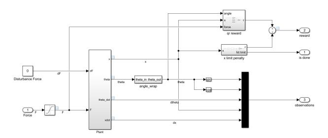
The cart-pole system is modeled using Simscape Multibody.
