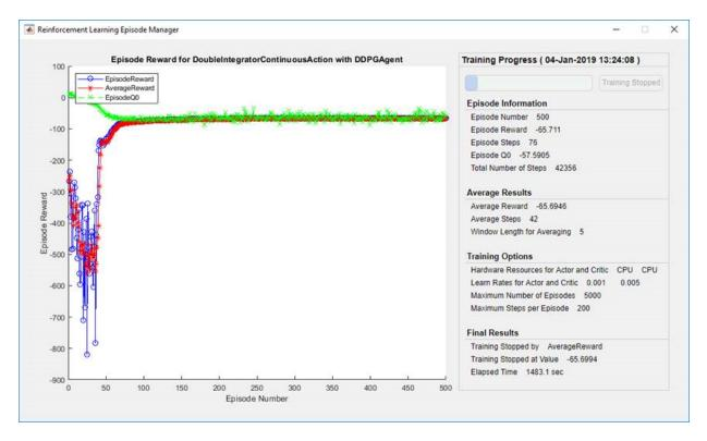
For agents with a critic, **Episode Q0** is the estimate of the discounted long-term reward at the start of each episode, given the initial observation of the environment. As training progresses, **Episode Q0** should approach the true discounted long-term reward if the critic is well-designed, as shown in the preceding figure.
